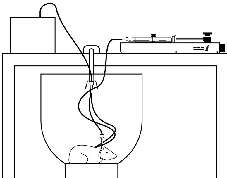
The MD probe was a DL-5 (MF-7051, BAS) (**F1b**) which contained one 5 cm fiber. This was implanted in a looped configuration making an implantable length of 2.5 cm. All probes were sterilized with ethylene oxide.
