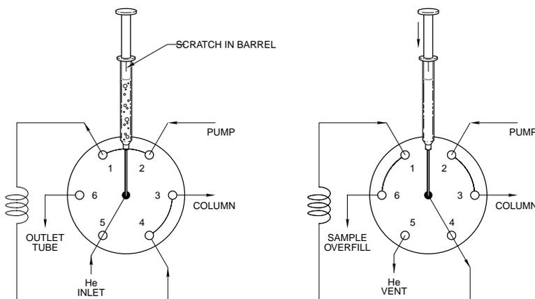
A 2-mL glass syringe with glass luer tip (#5006, Popper and Sons) was used to deoxygenate and inject the sample. A 2-cm-long scratch was made with a file, along the inside of the barrel where the plunger enters. The scratch allows the gas to escape when the plunger is pulled most of the way back. When you depress the plunger to inject the sample, it passes the scratched region and then seals normally.
