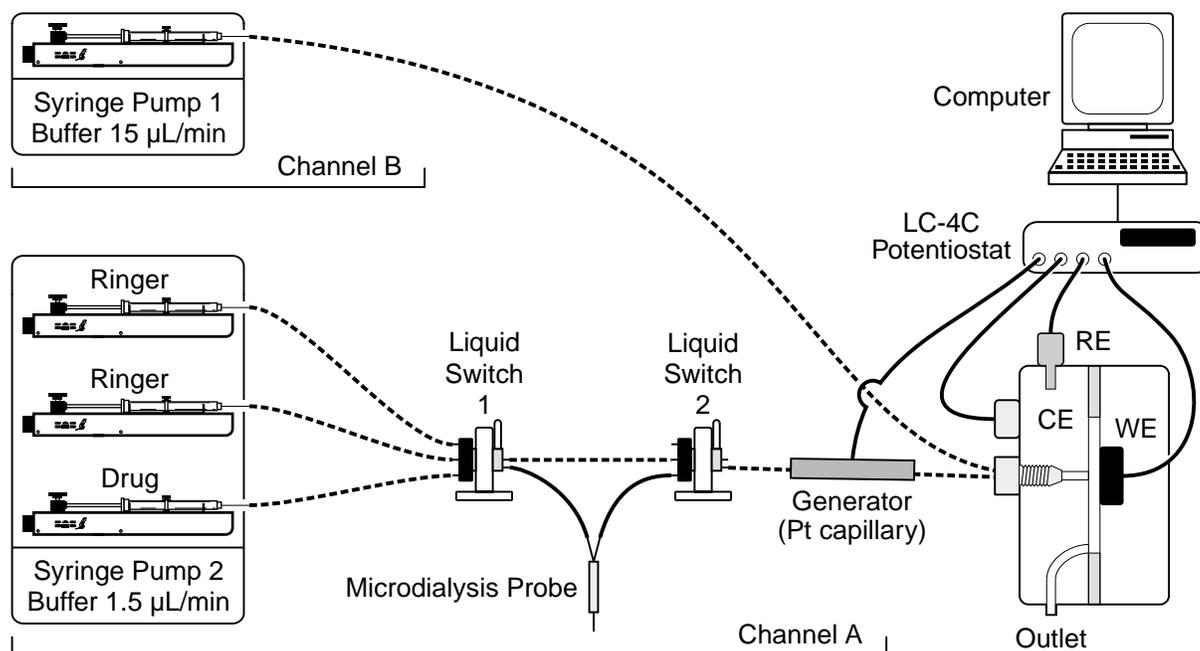
A. Channel B was blocked. Standard solutions of glucose and/or other drugs or samples were included/removed from the system by liquid switch 1 (**F1**). A three-point calibration curve was determined for the concentration of glucose vs. the current generated. Using a fast calibration method, a three-point standard curve could be performed in less than 30 minutes and pump noise was minimal.
