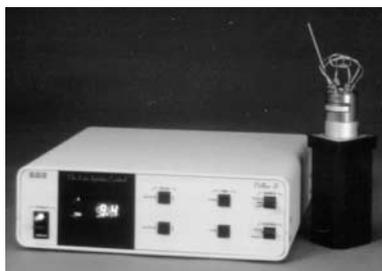
The dialysate collected in vials is neither contaminated nor diluted by LC mobile phase. The Honey-Comb advances to a new vial after receiving a signal from the Pollen-8.
