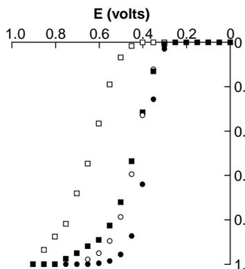
potential should be set to a value well positive of the observed half-wave potential of the analyte of interest to obtain maximum sensitivity (current per unit change in concentration).
