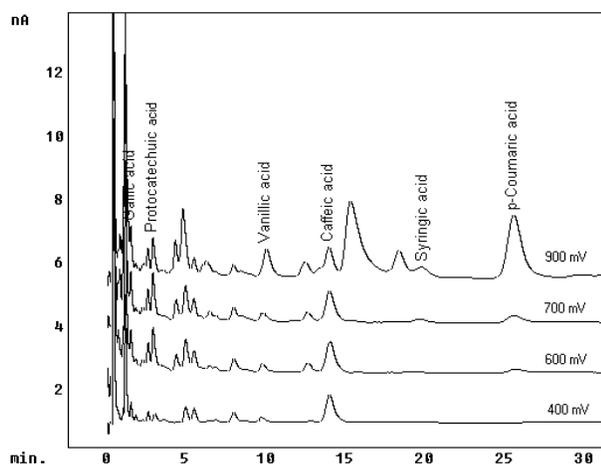
glassy carbon working electrodes in the arc configuration (see **F3**). For the first injection, the detectors were set to 300, 350, 400, and 450 mV (vs. Ag/AgCl). The detectors were reset to 500, 550, 600, and 650 mV for the second injection, and 700, 750, 800,
