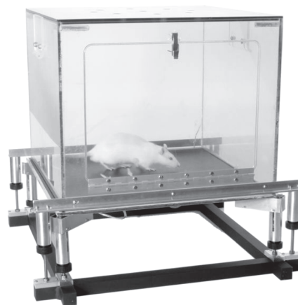
F2. The Force Plate Actimeter is enclosed by a ventilated sound-attenuating chamber and uses a proprietary interface to communicate with the FPA software.
